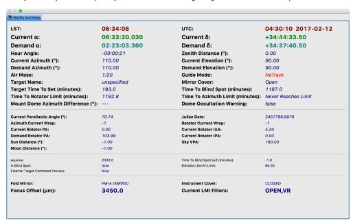
The majority of data comes from TCS Public Status packet which is published by the TCS at 1Hz. Additionally some information is provided by the AOS and DCS. This view is used by several LOUIs and there is very little customization for different instruments. Currently the "LMI Current Filters" field is only populated in the LMI LOUI.
