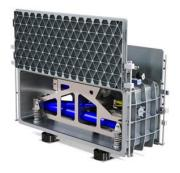
The EXPRES spectrograph structure. The outer vacuum enclosure maintains the spectrograph in a vacuum at better than 0.01 mBar, and using radiation shields and insulation maintains the temperature to better than 1 mK. The optics support structure visible inside the chamber maintains precise alignment of the optics and is mounted on a suspension to isolate it from mechanical vibrations. Removable panels allow easy access to the spectrograph for maintenance.
