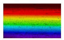
The white pupil design has three resolution modes: R = 30000, 45000, 60000 and we obtained the first light solar spectrum (5-second exposure) by running an optical fiber down the hall and holding it out the window! The image above shows the extracted 2-d spectrum and the plot on the one below shows the sodium doublet in all 3 resolution modes.
