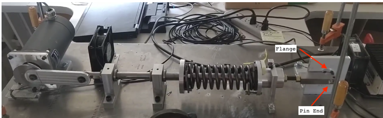
Figure 6. The jig set up for fatigue testing of the pins. The pin is on the right. The pin end is visible within the clamp, and part of the pin flange can be seen above the body of the clamp. 13
