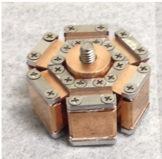
Figure 5. Flexible cold strap between cooler 1 and the rigid internal cold strap leading to the detector. The 8-32 screw in the center indicates the scale of the image.
