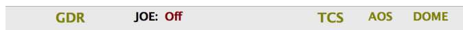
Figure 7: The Status Bar is located across the bottom of the NIHTS LOUI. Here, you can see the status of TCS, AOS, the dome, JOE, and the guider.
