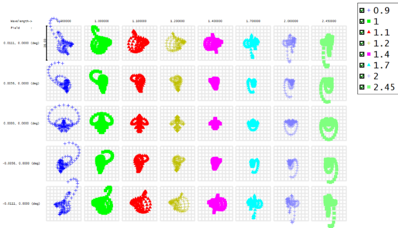
Figure 2. Spot diagrams for 5 fields (vertical) along the slit with the field center in the middle row and 8 wavelengths (horizontal) with 0.9 microns at the left and 2.4 microns at the right. The edge fields are 40" from field center and the intermediate fields are 20". The box size for each spot is 36 microns, about 2 pixels on the detector.
