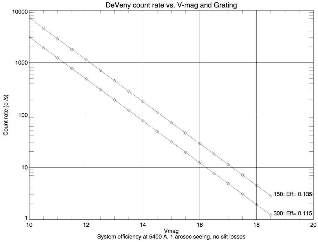
Figure E2. Count rate (e-/s) vs. V-mag and grating, at 5400 Å system efficiency.
