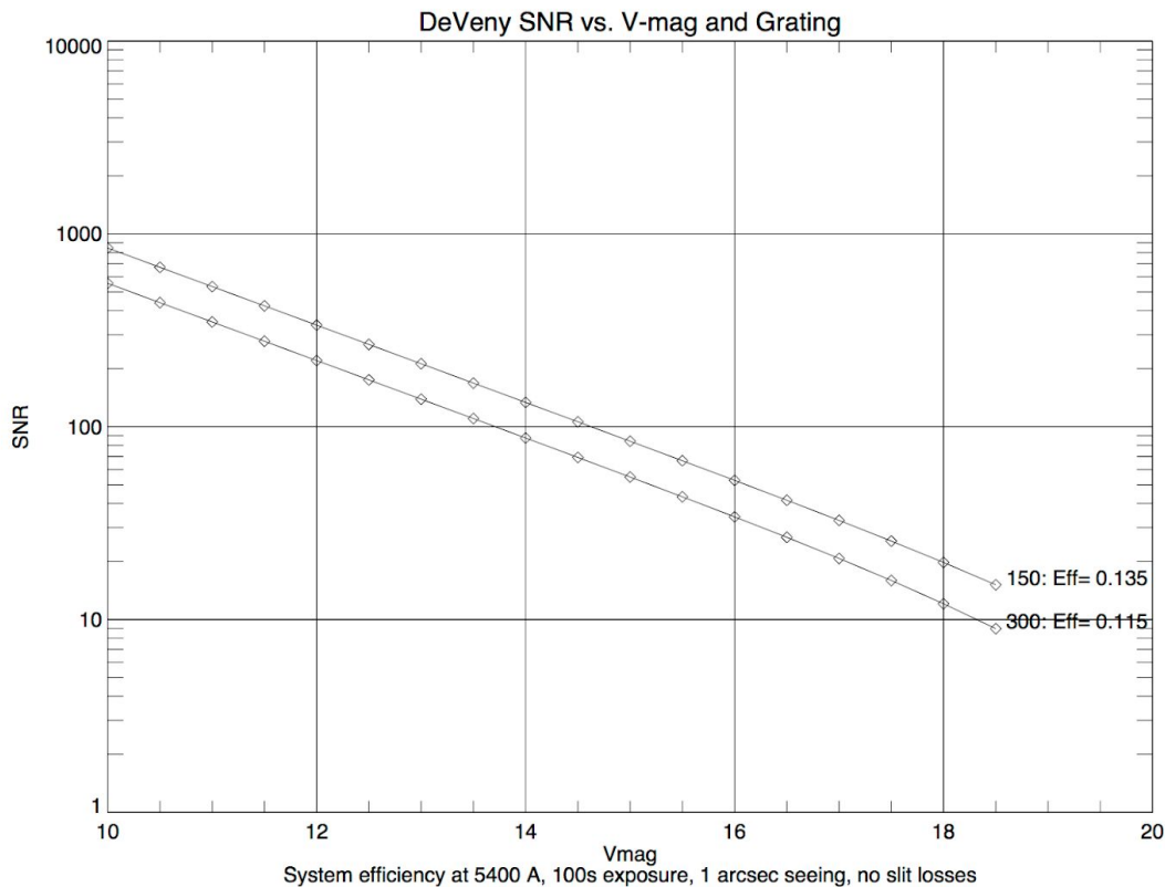
Figure E1. SNR vs. V-mag and grating, at 5400 Å system efficiency and 100 s exposure time.
