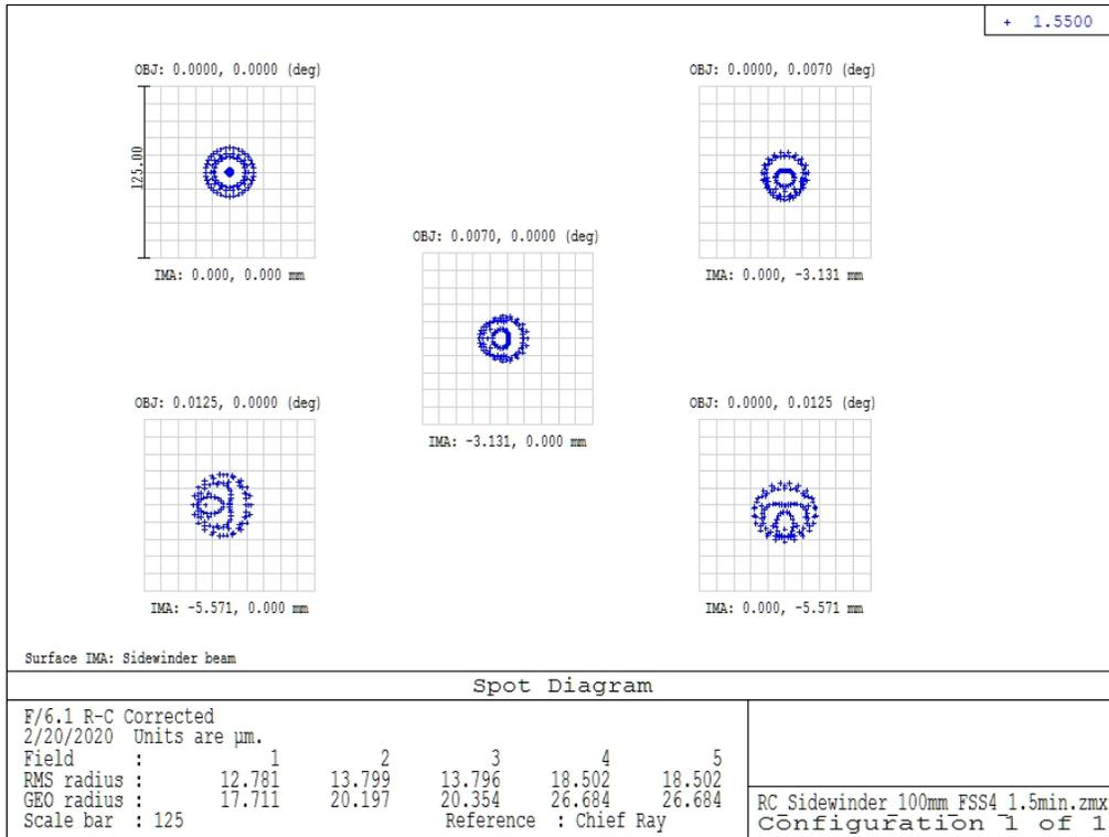
Figure 2. Spot diagrams for a 1:1 f/6.1 periscope relay. The field angles are  $[0, 0.007^\circ, 0.0125^\circ]=[0, 122\mu\text{rad}, 218\mu\text{rad}]$ . Box size is  $125\mu\text{m}$ , or  $1''$ .
