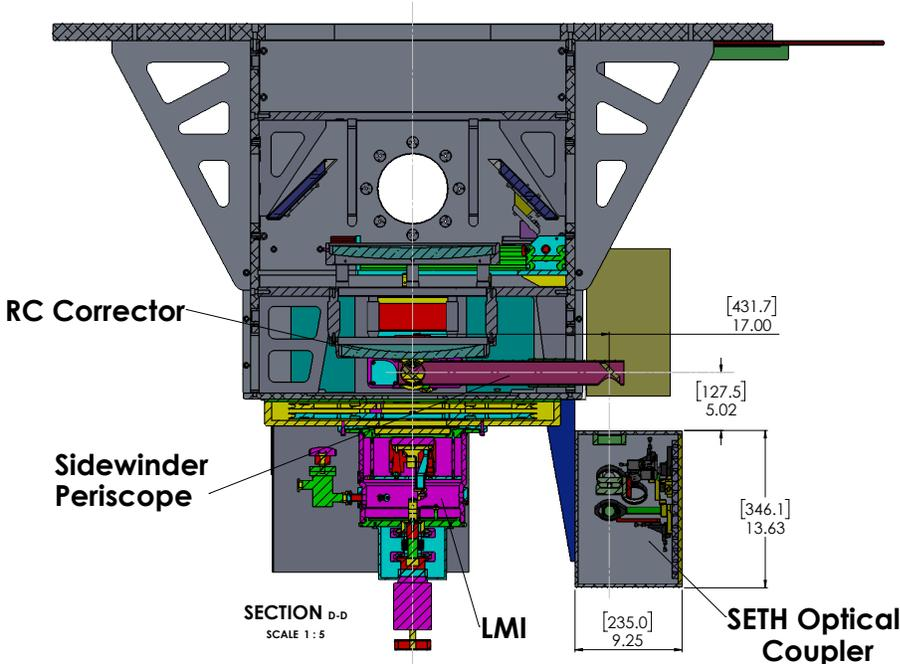
Figure 6. Cross section of the cube sidewinder-SOC installation and facility instrumentation. Dimensions are [mm] and inches.
