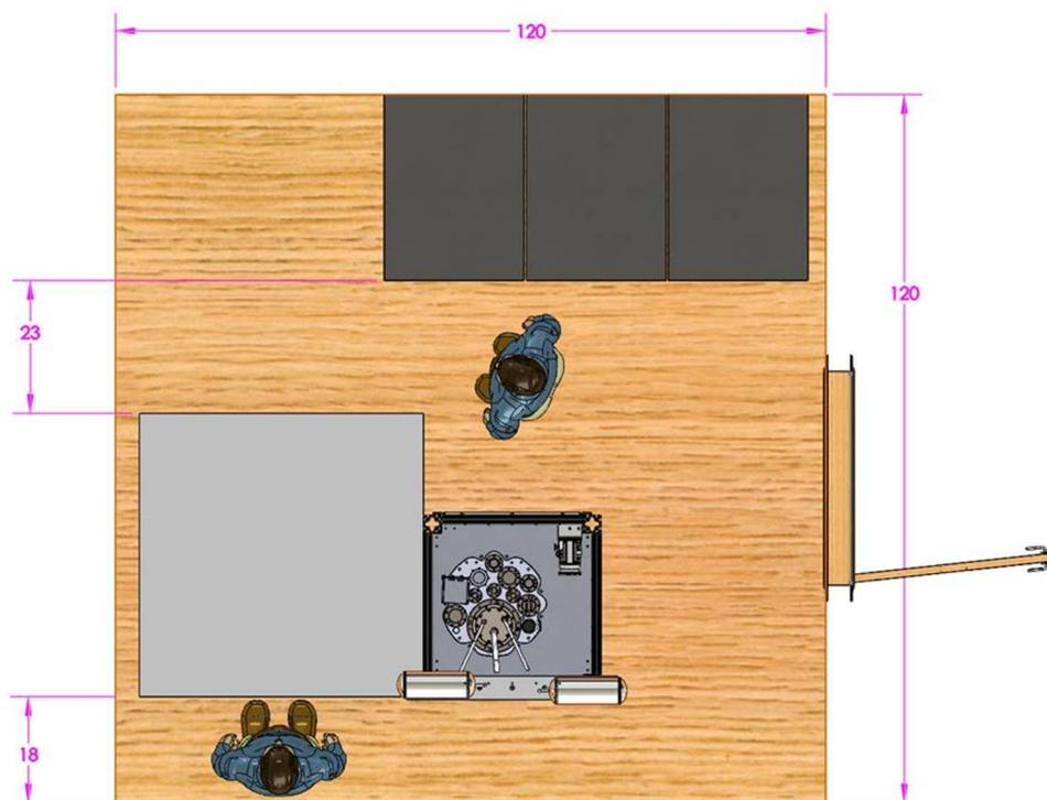
Figure 8. Internal view of the proposed Mezzanine Enclosure. Dimensions are inches.
