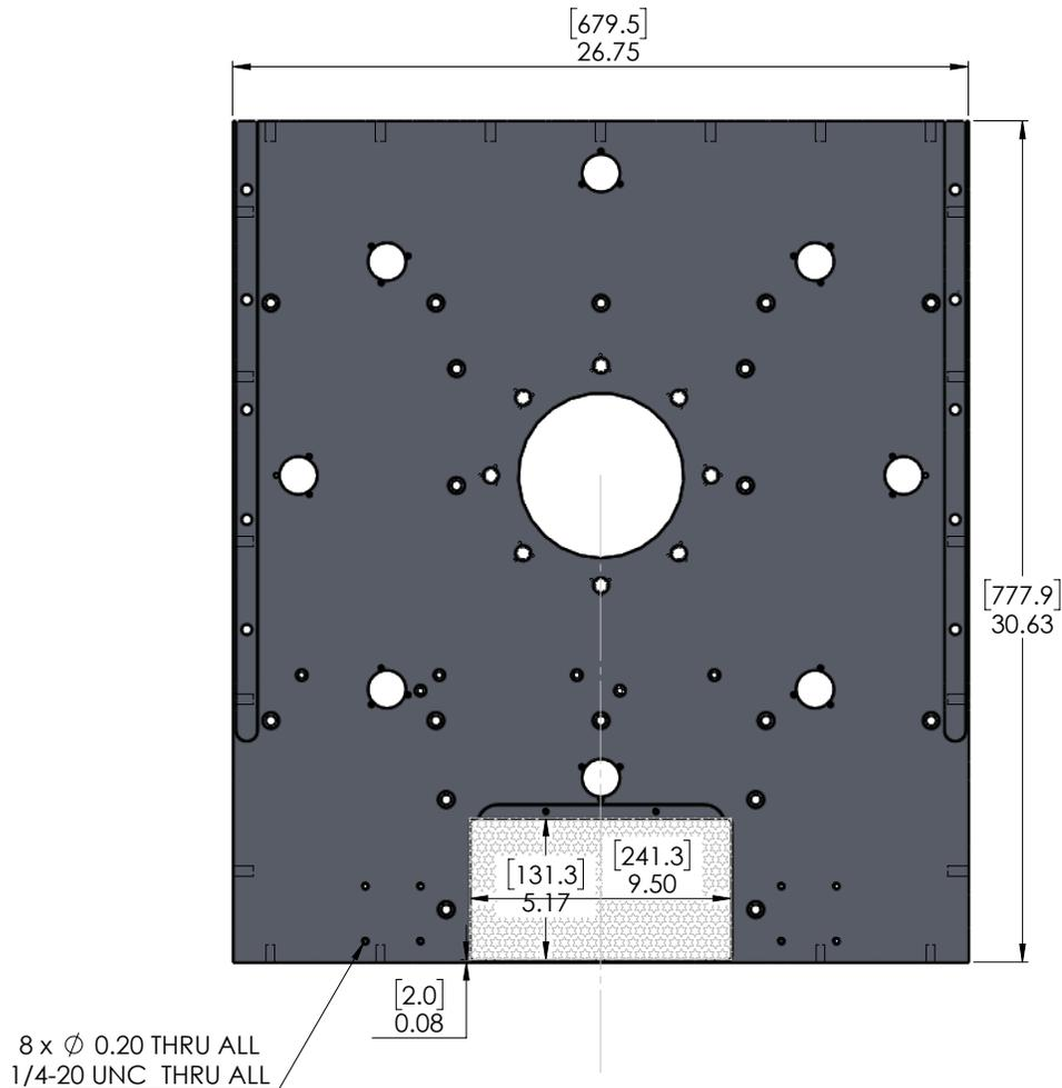
Figure 4. Cube A-side plate modifications, including removal of the hatched area and the addition of tapped holes. Dimensions are [mm] and inches; hole callout dimensions are inches.
