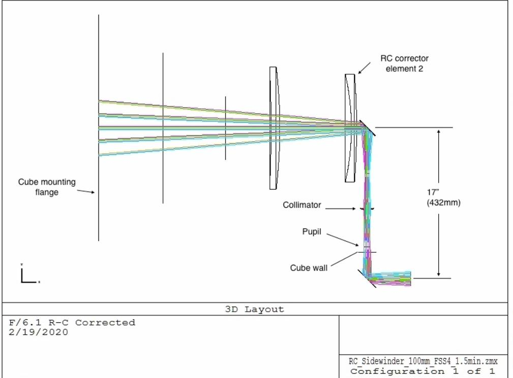
Figure 1. Sidewinder periscope and instrument cube optical layout.
