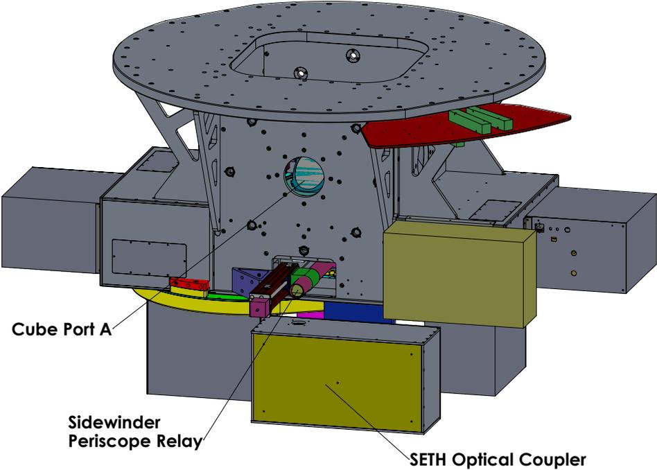
Figure 5. Sidewinder periscope relay and SETH optical coupler installation on the cube Port-A side.
