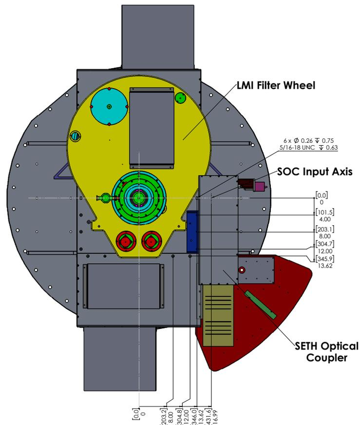
Figure 7. Position of the SETH optical coupler and a model mounting bracket with details of existing tapped mounting holes. Dimensions are [mm] and inches; hole callout dimensions are inches.
