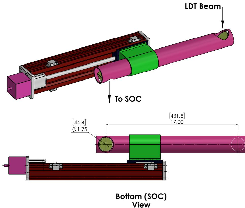
Figure 3. Sidewinder periscope concept assembly. Dimensions are [mm] and inches.
